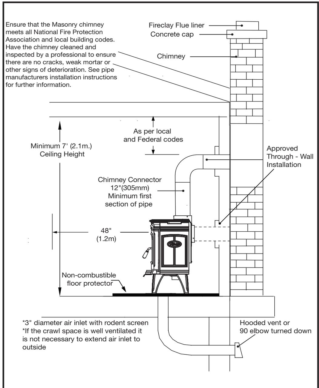
Figure 17: Alt 1.2 Venting to a masonry chimney.
