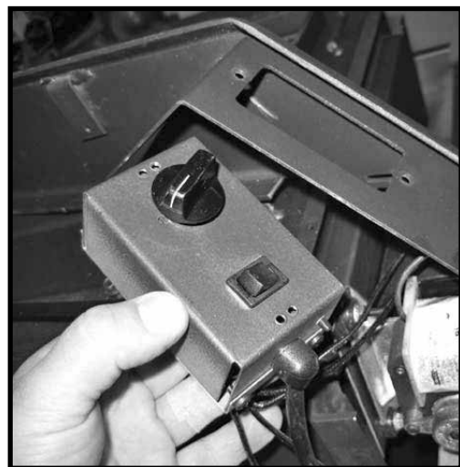
Figure 17: Removing speed control assembly.
