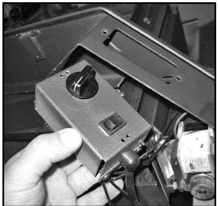
Figure 24: Removing speed control assy.
