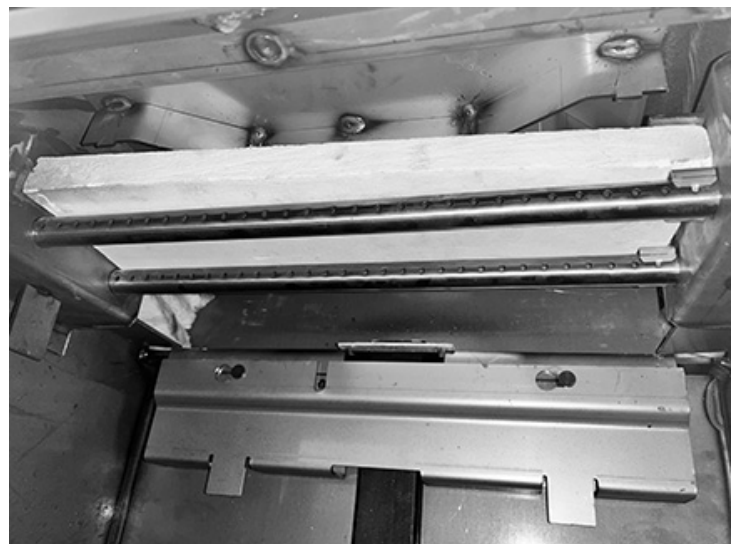
Figure 4: Baffle board installed.
