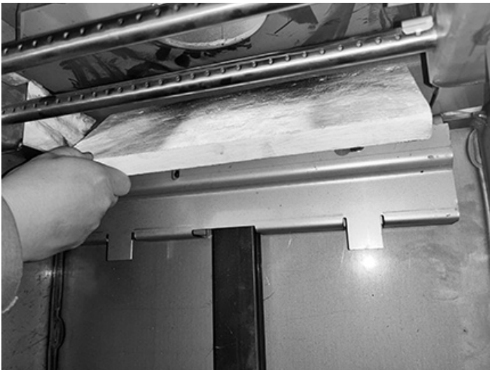
Figure 3: Baffle board removal.
