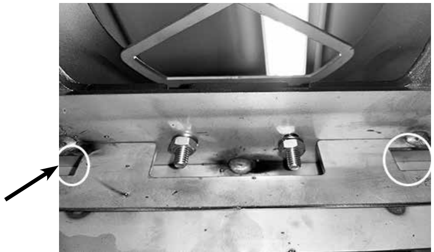
Figure 10: Front mounting slots for Flue Gas Agitator.
