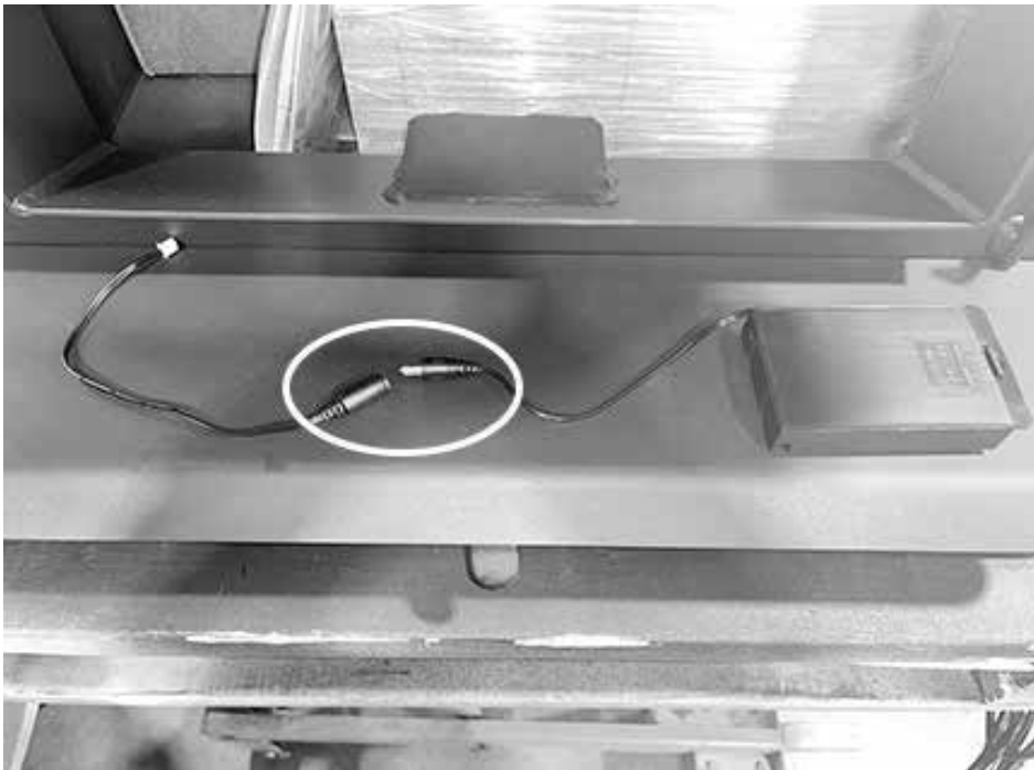
Figure 20: Remove barrel jack extension wire.
