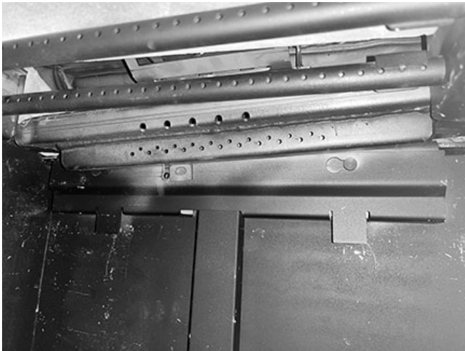
Figure 8: Remove rear baffle.
