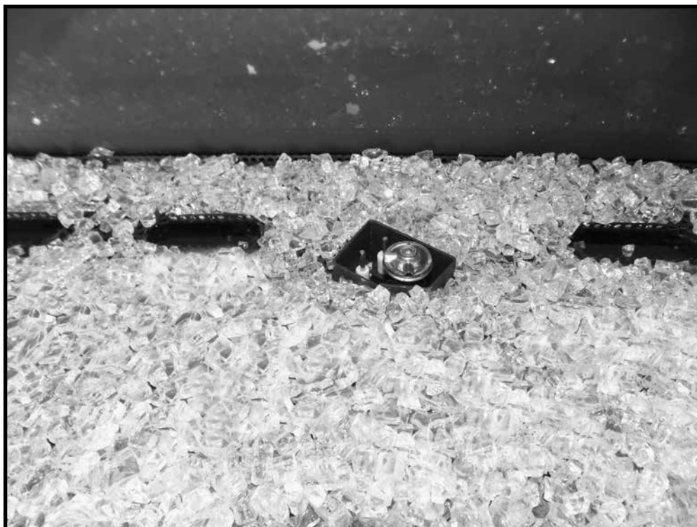
Figure 53: Glass media installation.
