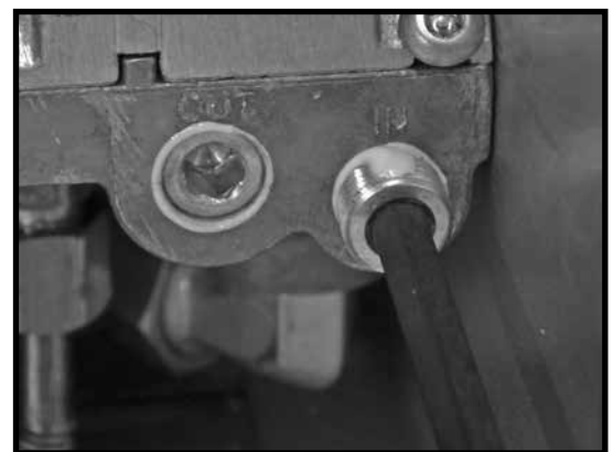
Figure 41: Testing port caps with thread sealant.
