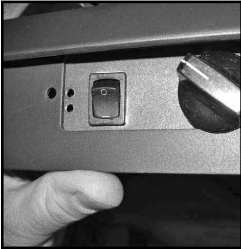
Figure 18: Reinstalling the Speed control assembly.
