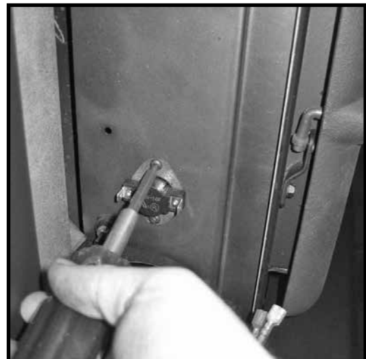
Figure 21: Relocating thermal switch to left side.
