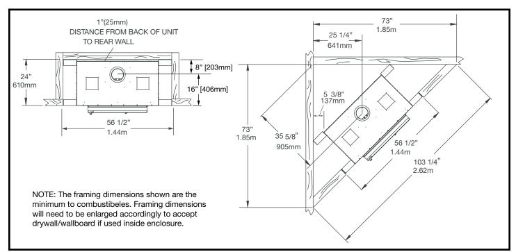
Figure 9: FP30 Framing dimensions. The top front framing must be built as shown, (Figure 10) with no wood framing directly in front of the chimney system
