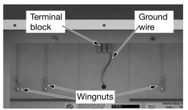
Figure 5: Terminal block, blower wingnuts and ground wire
