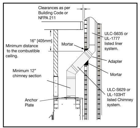
Figure 15: FP Masonry Installation.
