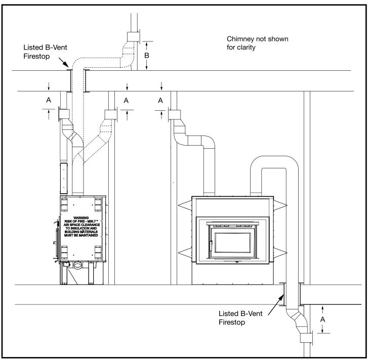
Figure 21: FP Remote heat duct Options.
