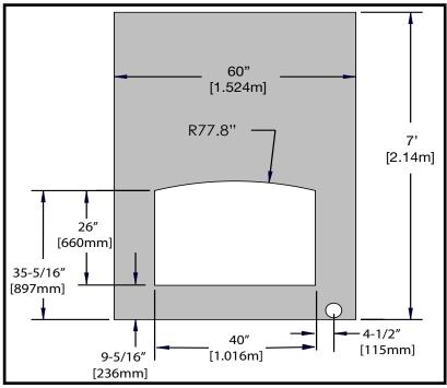
NOTE: the dimensions shown here are from the bottom of the unit. If the unit is raised, add the height to the bottom dimensions.
