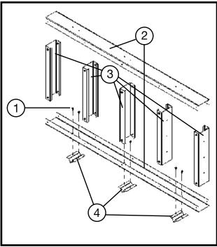
Figure 11: Framing kit parts.
