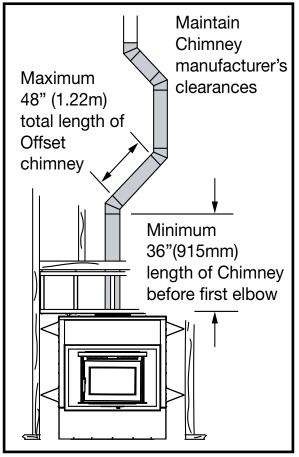
Figure 14: FP Offset Installation.
