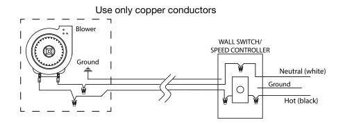
Figure 29: WODC.RHkit wiring diagram.
