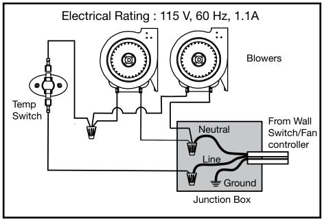
Figure 19: FP Wiring Diagraml.
