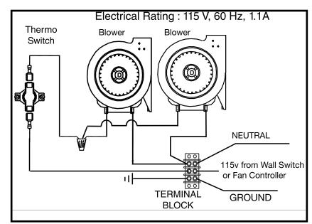
Figure 7: Electrical diagram
