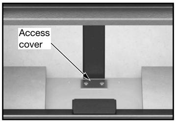
Figure 2: Secondary Airbox clean out cover.
